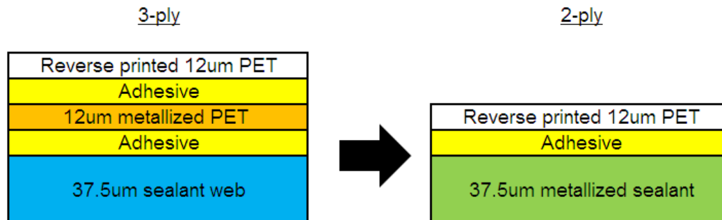
Figure 1: Comparison of 3-ply vs. 2-ply Structures for Stand-up Pouches
