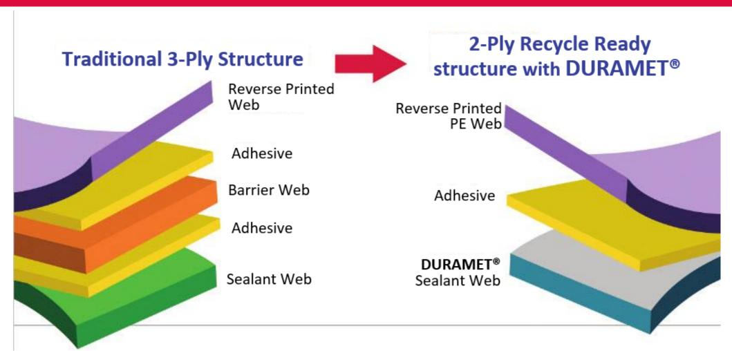
◆ DURAMET® top-coating applied on recyclable film substrates delivers high barrier recycle ready packaging structures.
